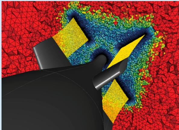
By using baffles (shown in yellow) with the T-Rex hybrid meshing technique, you can cluster cells around thin surfaces or flow features. Shown above is wake clustering behind the tailplanes of the SUBOFF benchmark submarine geometry.
