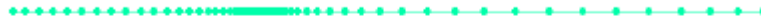
Figure 4.2: Grid points on the connectors are clustered towards the location of the backward step.
